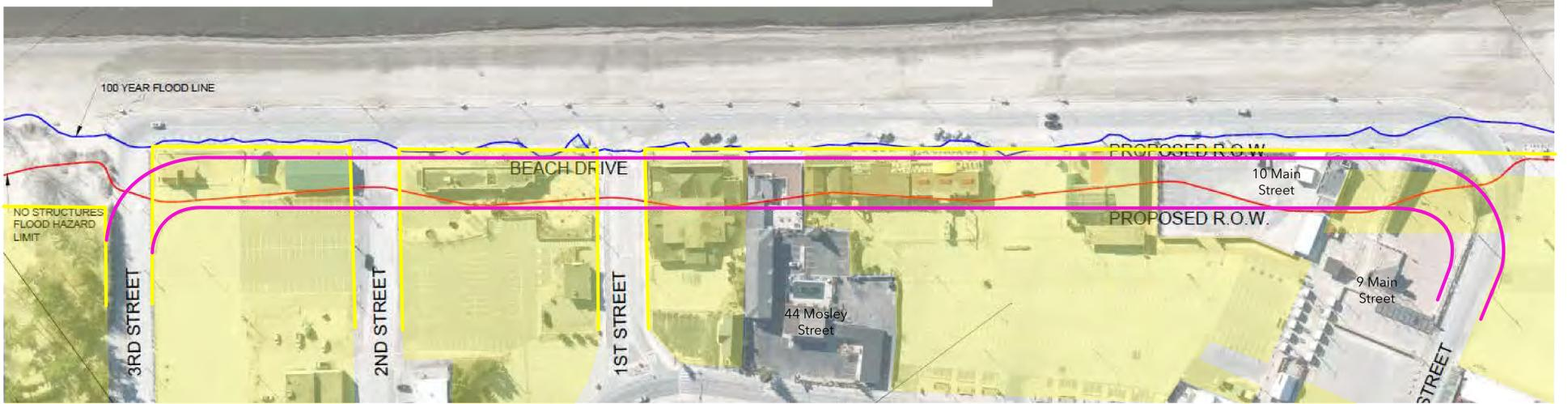
Option 3: No Structure Flood Hazard Limit (shift 46 metres south)
