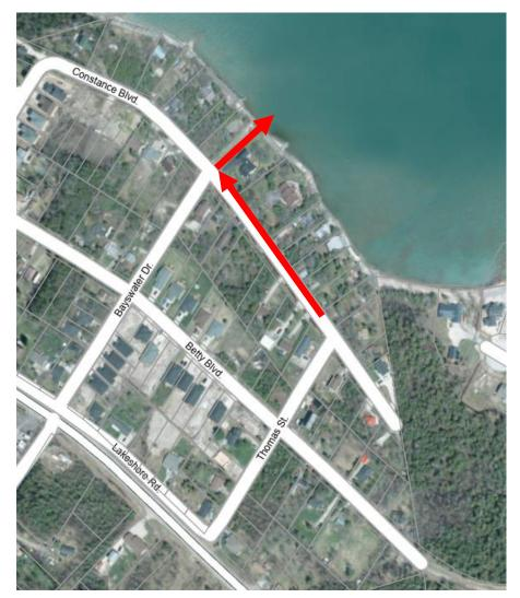
Option 3 - Increase Capacity of Constance Boulevard Ditch to Outlet North of Bayswater Drive
